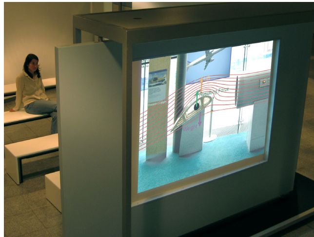
Figure 4. Student following a classmate's view of an interactive exhibit (real aerofoil augmented with virtual airflow and force vectors).
