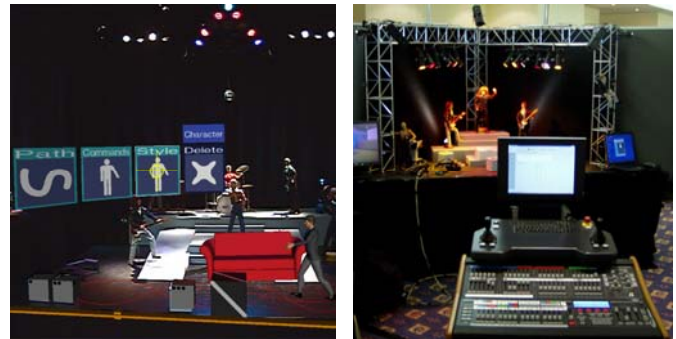
Fig. 7. 3D menu, view-pointer and tangible unit as user interface elements of the Mixed Reality Stage (left), stage control board and lighting board in front of the model stage (right)
